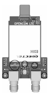
Please note that a GPS antenna is **not included** with the device, and one can only be connected with the top cover disassembled.
